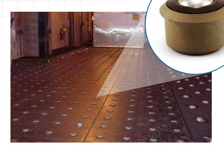
RBC's patented EverGlide T-Ball™ is designed to fit in industry standard holes of 1¾". Also features 0.54" exposed height for easy drop-in back replacement on existing ball transfer decks.
